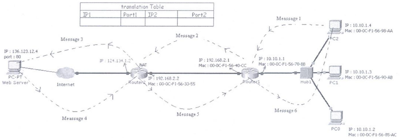
Suppose that the PC2 want to send a web request to the web server (136.123.12.4), the browser is running in port 1234, the web server will reply with a web response to the PC2.
